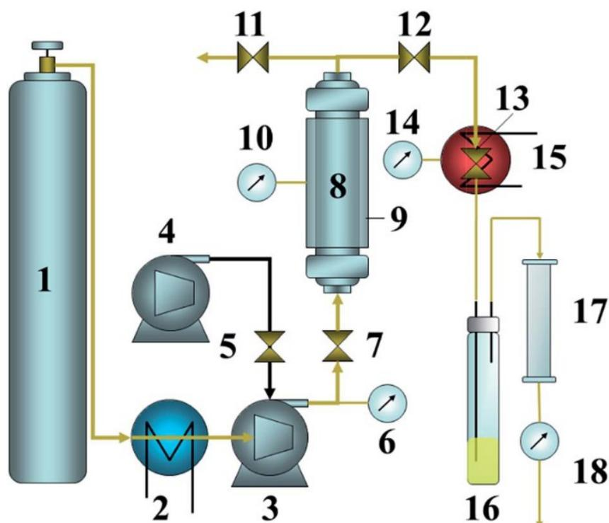
Key: 1 - CO<sub>2</sub> cylinder; 2 - cooling bath; 3 - air driven fluid pump (gas booster pump); 4 - air compressor; 5 - air regulator; 6 - CO<sub>2</sub> pressure; 7 - inlet valve; 8 - extraction vessel; 9 - heating jacket; 10 - vessel heat; 11 - vent valve; 12 - outlet valve; 13 - flow valve; 14 - valve heat; 15 - heating jacket; 16 - collecting vial, 17 - alumina filter; 18 - gas flow meter
