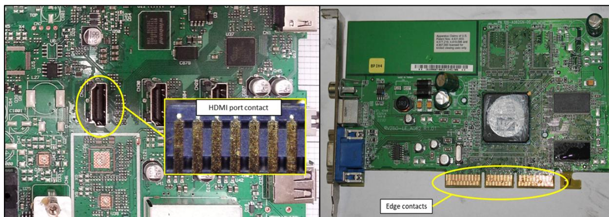
Figure 15: Photograph of the coated Au on the surface of a mobile phone PCB.
